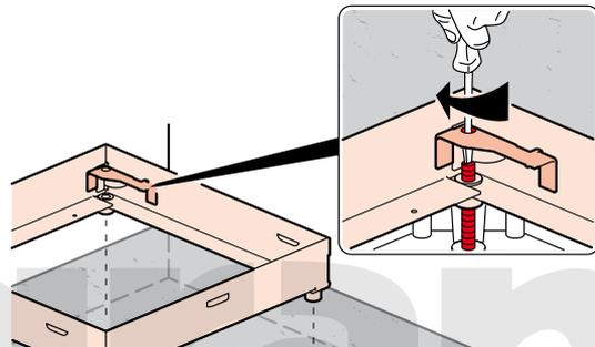
Make a rough adjustment to finished floor level by turning threaded rods in each corner with a screw driver
