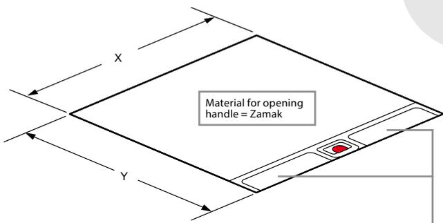
Full metal rigid cable exits: Maximum cable capacity 4 cables Ø 7 mm + 3 cables Ø 11 mm Provides maximum protection for cables and strength
