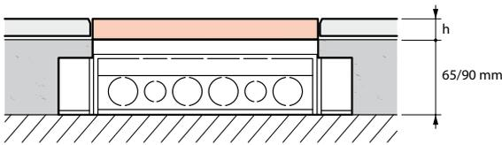
Total screed thickness has to be between 65 and 90 mm
