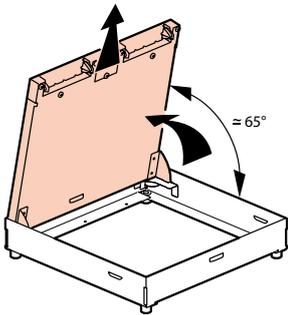
To remove the lid from the trim, hold it under an angle of approximately 65° and pull it out
