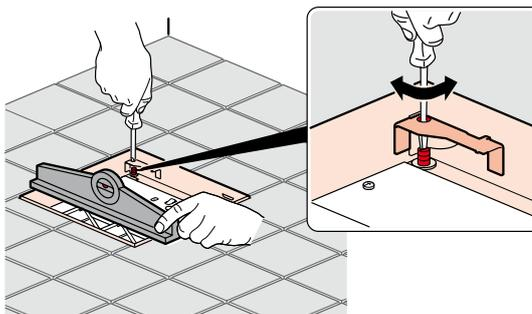
Make final adjustment to finished floor level by turning threaded rods in each corner with a screw driver
