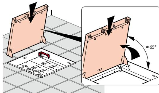
Push the lid back in place by holding it under an angle of approximately 65°
