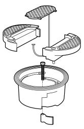
3 piece GRP top, with removable section to allow passage of cables.
