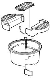
3 piece GRP top, with removable section to allow passage of cables.
