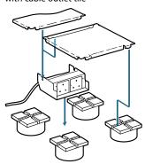
Fully submerged Arteor data unit with cable outlet
