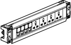
Embed the complete block in the wall and screw until the module gets fixed.
