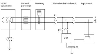
P1: main protection of the installation SPD: surge protective device with Uc 440 V (Uc
