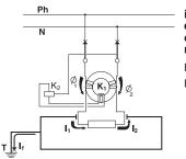
Therefore no current is induced in coil K<sub>1</sub>, and coil K<sub>2</sub> is not excited. The contacts do not open. The equipment operates normally
