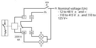
Equipped with a signalling contact which indicates tripping of the shunt trip and automatically breaks the coil. Min. and max. voltage: 0.7 to 1.1 Un Tripping time: less than 20 ms Power consumption: at 1.1 x 48 V = 121 VA at 1.1 x 415 V = 127 VA
