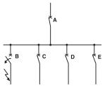
Discrimination between A and B is said to be "total" if it is provided up to the value of the maximum prospective short-circuit at the point at which B is installed. By extension, in the tables on the
