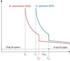
$I_{\mbox{\tiny SCB}}$  : maximum short-circuit at the point at which MCB B is installed
