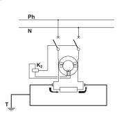
.. coil K<sub>2</sub> is excited, the contacts open and the equipment is automatically switched OFF
