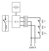
Signalling auxiliaries Umin.: 24 V  $\pm$  /= and Imin.: 5 mA
