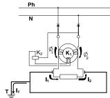
Therefore no current is induced in coil K<sub>1</sub>, and coil K<sub>2</sub> is not excited. The contacts do not open. The equipment operates normally
