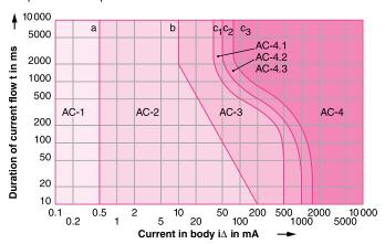
$i\Delta$ : current flowing through body. t: time taken for current to pass through body.
