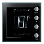
After a few seconds the new set-point is saved and the measured temperature appears.
