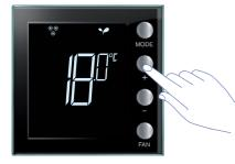
The symbol of the new mode appears and the set temperature flashes (thermometer symbol off). Use + and - to change the set-point.
