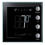
The display shows the 0 symbol and the value set: 7 °C if heating is on; 35 °C if cooling is on.
