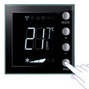
Press FAN to set the fan speed at the desired level.
