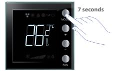
To switch from heating to cooling, and vice versa, press MODE for more than 7 seconds.
