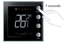
To switch from heating to cooling and vice versa press MODE for more than 7 seconds.
