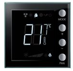
After a few seconds the new set-point is saved and the measured temperature appears. In this example the set temperature is higher than the measured temperature, therefore also the heating on indicator will come on **(s)**.
