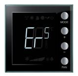
**NOTE:** if ER4 or a temperature very different from the one felt are displayed, or after the first installation, wait at least 5 hours before checking the operation again. If the problem continues, contact a trusted technician.
