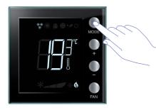
To switch from normal operation to Antifreeze (or thermal protection) press the MODE key.
