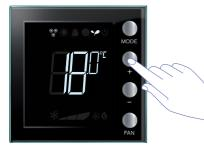
The symbol of the new mode appears and the set temperature flashes (thermometer symbol off). Use + and - to change the set-point.).
