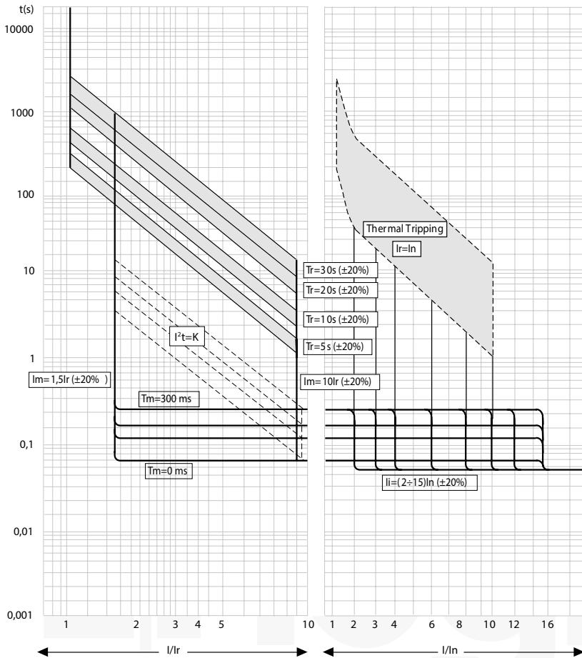
If short-circuit current is higher than  $lcw$  value or  $li$  is setted at  $lcw$  position, tripping time is equal to 30ms
