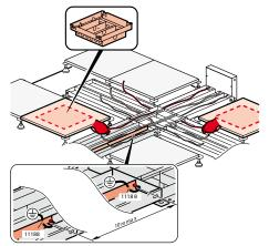
Cut raised access floor tiles according to backbox size and earth the system (minimum every 10 meters)
