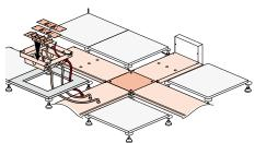
On trunking, remove knockouts to fit flexible conduit. Fix the wiring accessory plates. Earth the system
