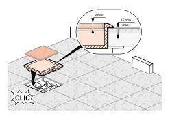
Fit the floor covering (carpet,...) and clip the lid and trim onto the backbox (push and fit principle)
