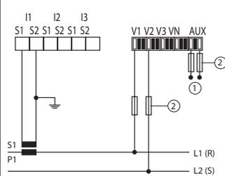
① Auxiliary power supply: 110 ... 400 VAC/120 ... 350 VDC
