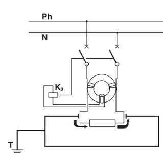
...coil  $K_2$  is excited, the contacts open and the equipment is automatically switched OFF
