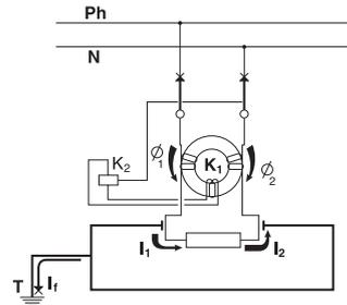
Therefore no current is induced in coil  $K_1$ , and coil  $K_2$  is not excited. The contacts do not open. The equipment operates normally
