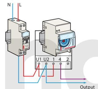
Output closing and breaking times are calculated based on the date, the actual time when the device was switched and on geographical coordinates of the actual location
