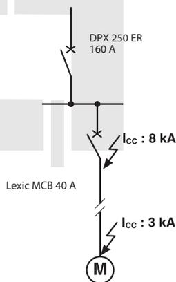
Since almost all faults occur during use, partial discrimination may be adequate if the discrimination limit is higher than the value of the maximum short-circuit which may occur at the point of use (or at the end of the trunking). This is referred to as "operating discrimination". This technique is very often adequate, more economical and less restricting in terms of implementation.
