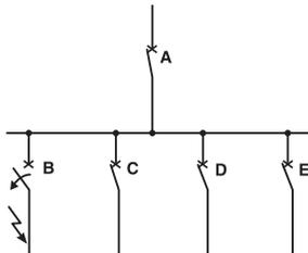
Discrimination between A and B is said to be "total" if it is provided up to the value of the maximum prospective short-circuit at the point at which B is installed.
