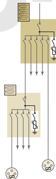
Effective protection against overvoltages cannot generally be assured with a single SPD if its protection level (Up) is greater than 1.2 kV (EN/IEC 62305 and TS/IEC 61643-12).
