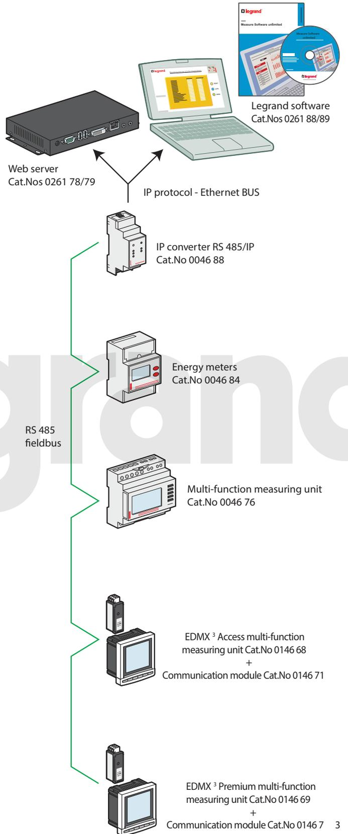
EDMX<sup>3</sup> Premium multi-function measuring unit Cat.No 0146 69 + Communication module Cat.No 0146 71 3
