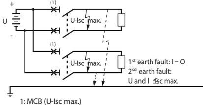
Example: isolated earth circuit /  $U = 48\text{ V}$  /  $I_{sc} = 4.5\text{ kA}$  /  $I_n = 40\text{ A}$
