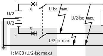
Example: circuit earthed via a middle point /  $U = 230\text{ V}$  /  $I_{sc} = 6\text{ kA}$  /  $I_n = 10\text{ A}$
