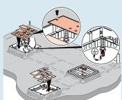
Connect wiring to accessory plates and them fix to the backbox. Finally, earth the system.
