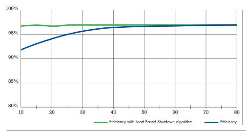
Load Based Shutdown algorithm optimizes the number of active modules to maximize system efficiency. This enables the UPS to adapt to load requirement, whilst keeping highest VFI protection.
