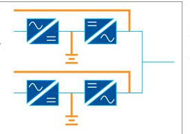
Each 333 kW module is equipped with a static bypass switch and a dedicated battery bank.
