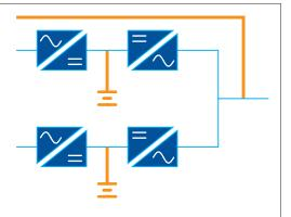
A central static bypass switch is fitted, sized for the whole UPS power. Each 333 kW module is equipped with a dedicated battery bank.
