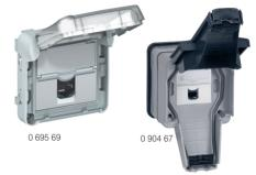
Sockets with LCS³ quick-fixing crimp connector. Take AWG 22 single-core cables up to AWG 26 and AWG 24 multicore cables. Contacts marked with dual colour code and wiring schemes T 568 A and T 568 B. Conforming to standards ISO/IEC 11801 Ed. 2.0, EN 50173-1 and TIA/EIA 568
